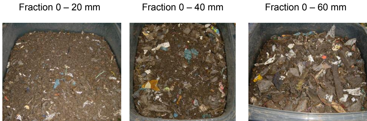
Figure 2 Sieve fractions of aerobic treatment in SHG (photogr. Ulrich Langer)
